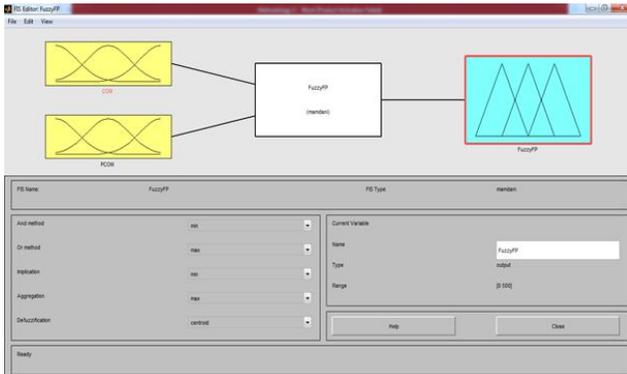
FIGURE.5 MAMDANI FIS DEVELOPED USING MATLAB.
